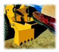
Safety and productivity is enhanced through features that include an operator-presence system that disengages the trencher if the operator leaves the controls, a trenching cleat that restricts rearward motion when trenching, and a minimal maintenance digging chain drive.
