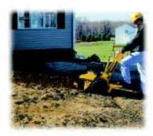
Trench a straight line and reduce physical labor with help from the patent-pending Vermeer ground-drive system. This system helps the operator create straight, uniform trenches while reducing the labor typically associated with operating small, non-propelled trenchers.
